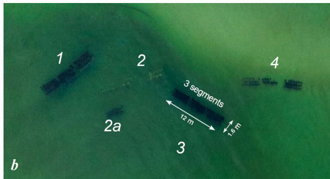
Fig. 3. Initial and final location of the “Grebенka” breakwater modules: a – initial (red lines) and final (blue lines) location of the modules (Google Maps image, 2021. https://www.google.ru/maps ); b – location of the “Grebенka” breakwater modules on 12 April 2023
