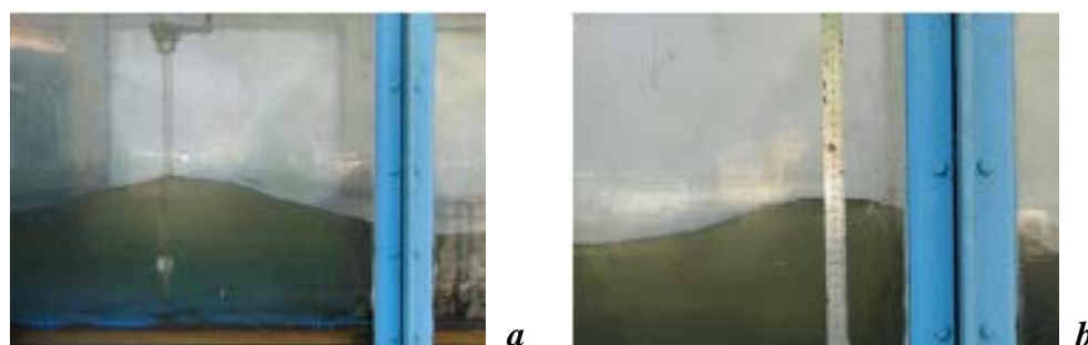
Fig. 1. Determination of wave heights on the model using capacitive wave recorders DUE (a) and a ruler (b)
