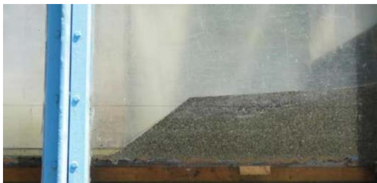
Fig. 4. Model of the initial backfill of the beach-forming material. The horizontal line shows the water level at high tide
