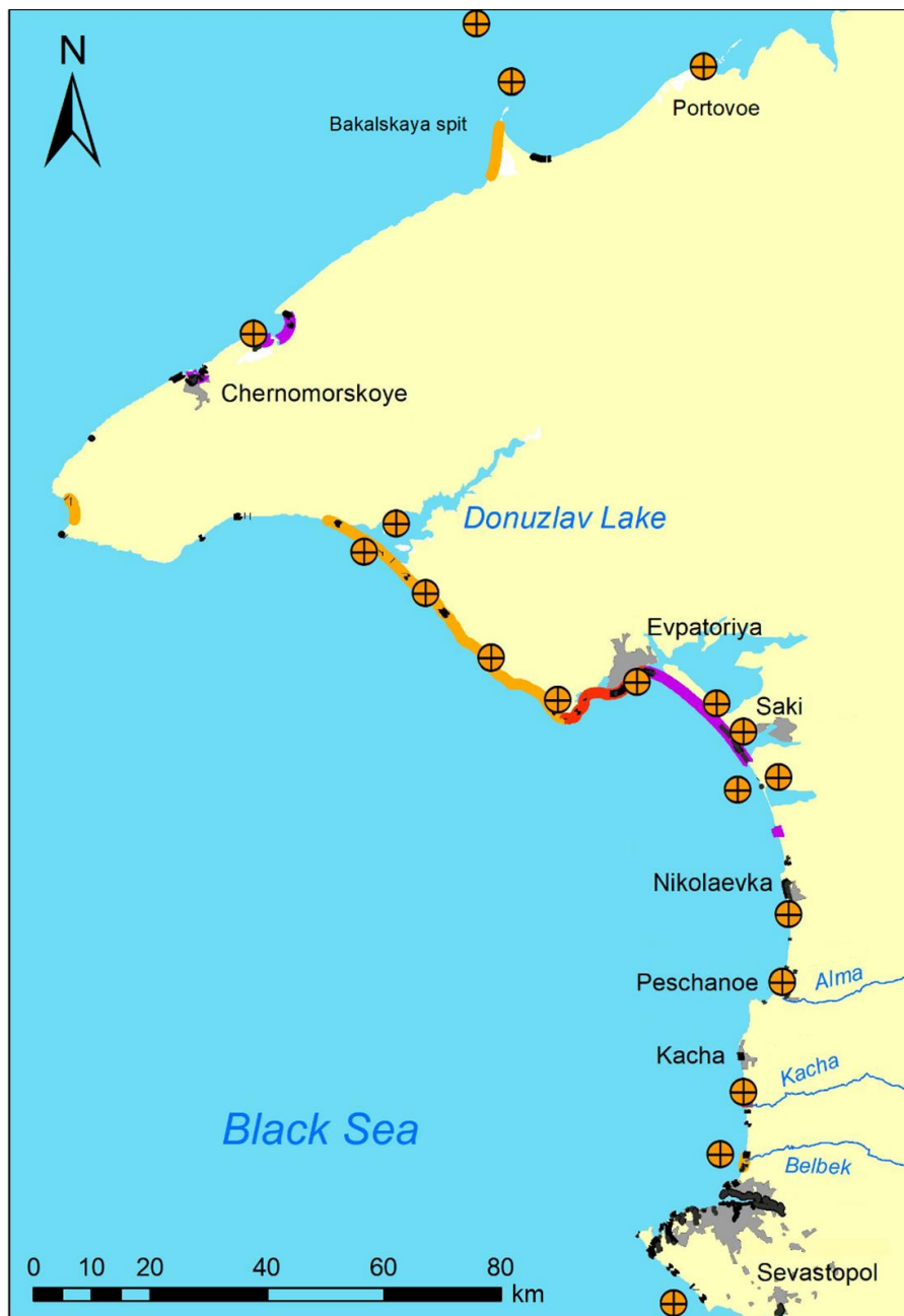
Fig. 2. Negative effect on lithodynamics of the coastal zone (slightly transformed dunes – orange lines, significantly transformed dunes – purple lines, destroyed dunes – red lines); circles – sand extraction on an industrial scale; black spots denote permanent facilities on the beaches
