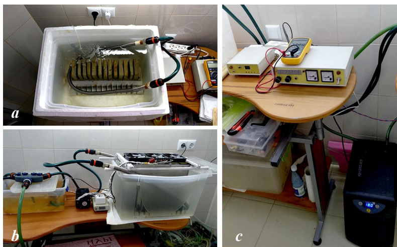
Fig. 1. Long-term laboratory experiment: a – control container (CC) with concrete and stainless steel plates; b – test container (TC) with the ultrasonic device (USD) and similar plates; c – devices for setting the time and power modes of USD operation ( top ) and HAILEA device for water cooling and temperature control ( bottom )
