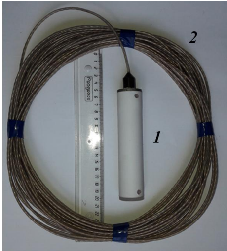
Fig. 1. Autonomous internal wave measurer: recording device – 1; line temperature sensor (LTS) 20 m long – 2
