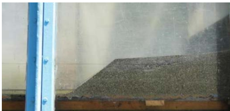
Fig. 4. Model of the initial backfill of the beach-forming material. The horizontal line shows the water level at high tide
